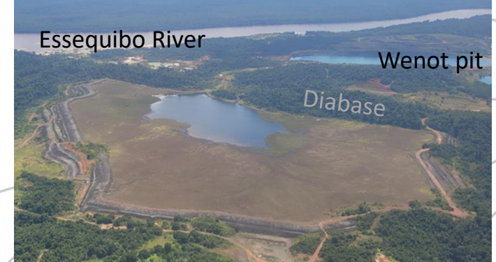
350 Acre Tailings Facility with excess capacity, configured for dam raises plus convenient alternative pit
