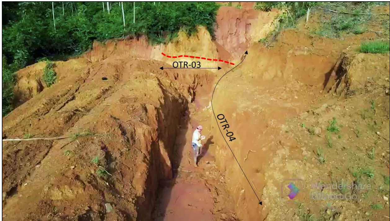
FIGURE 9.16 OTR-03 AND OTR-04 SAMPLE LOCATION LOOKING EAST, MAIN QUARTZ VEIN IN RED DOTTED LINE
