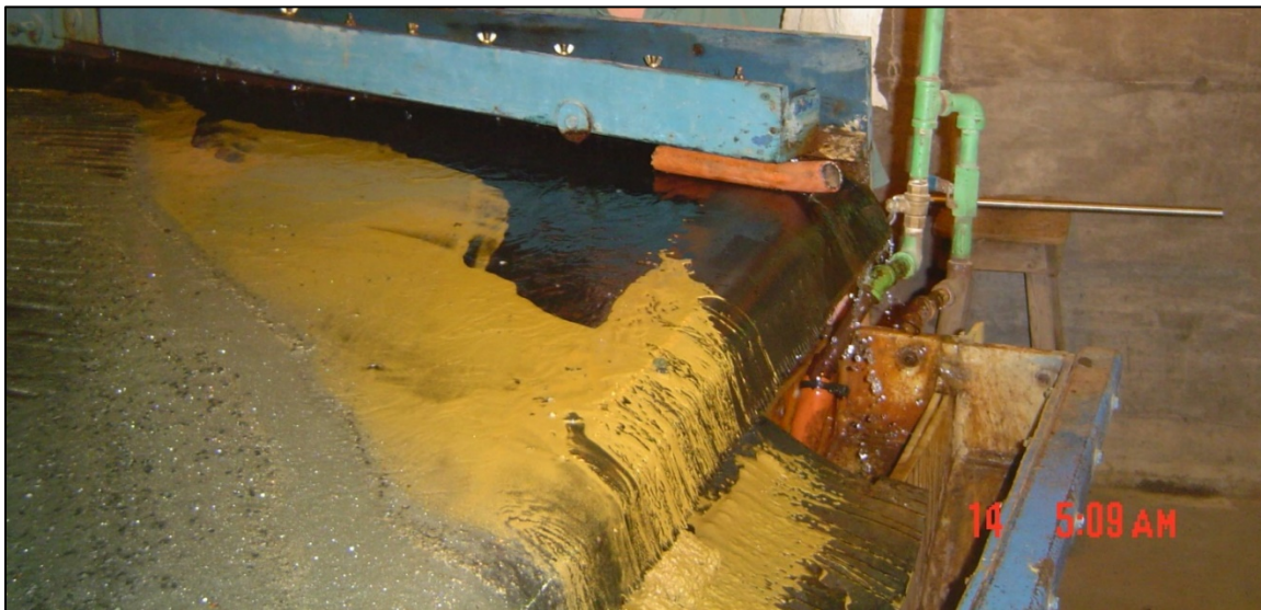
FIGURE 13.2 GOLD CONCENTRATION ON SHAKING TABLE
