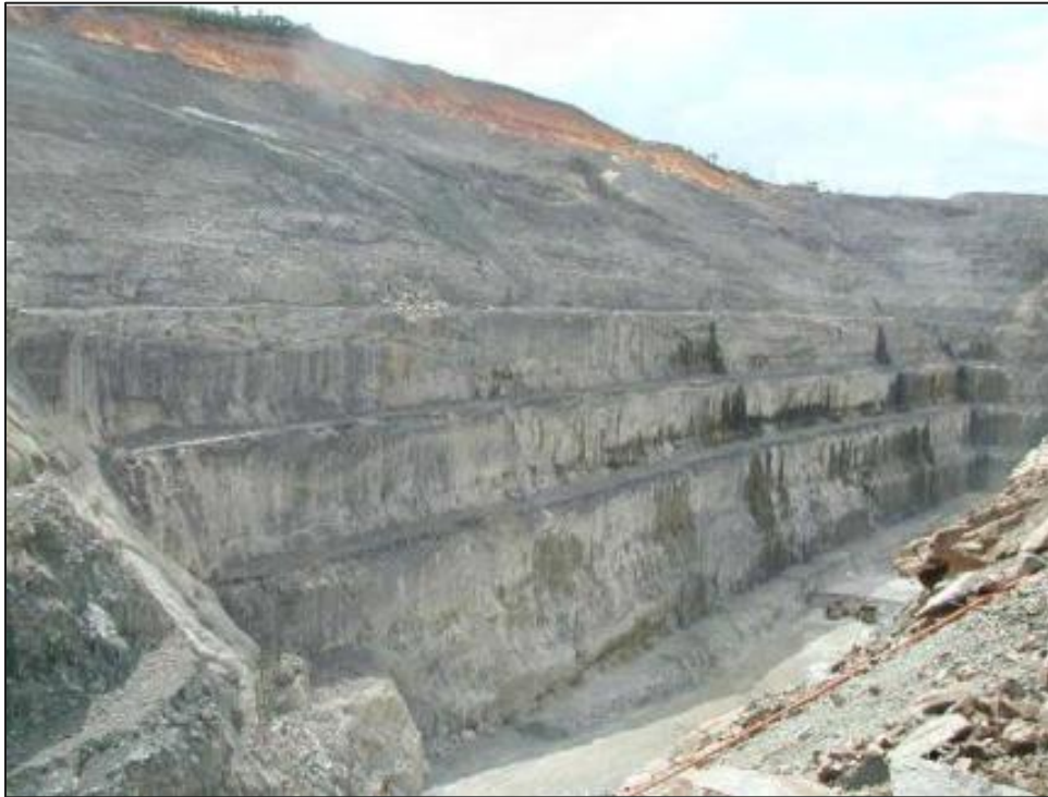
Figure 16-2: Steep Footwall of Wenot Pit Developed in Competent Bedrock Below Saprolite (North side)
