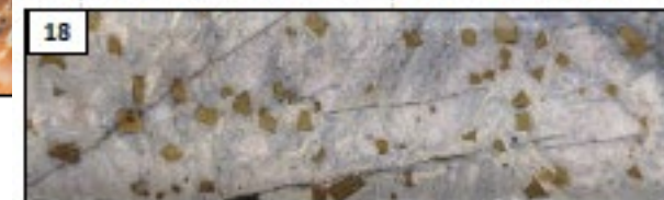
Completely altered quartz-sericite-pyrite-ankerite-albite zone
