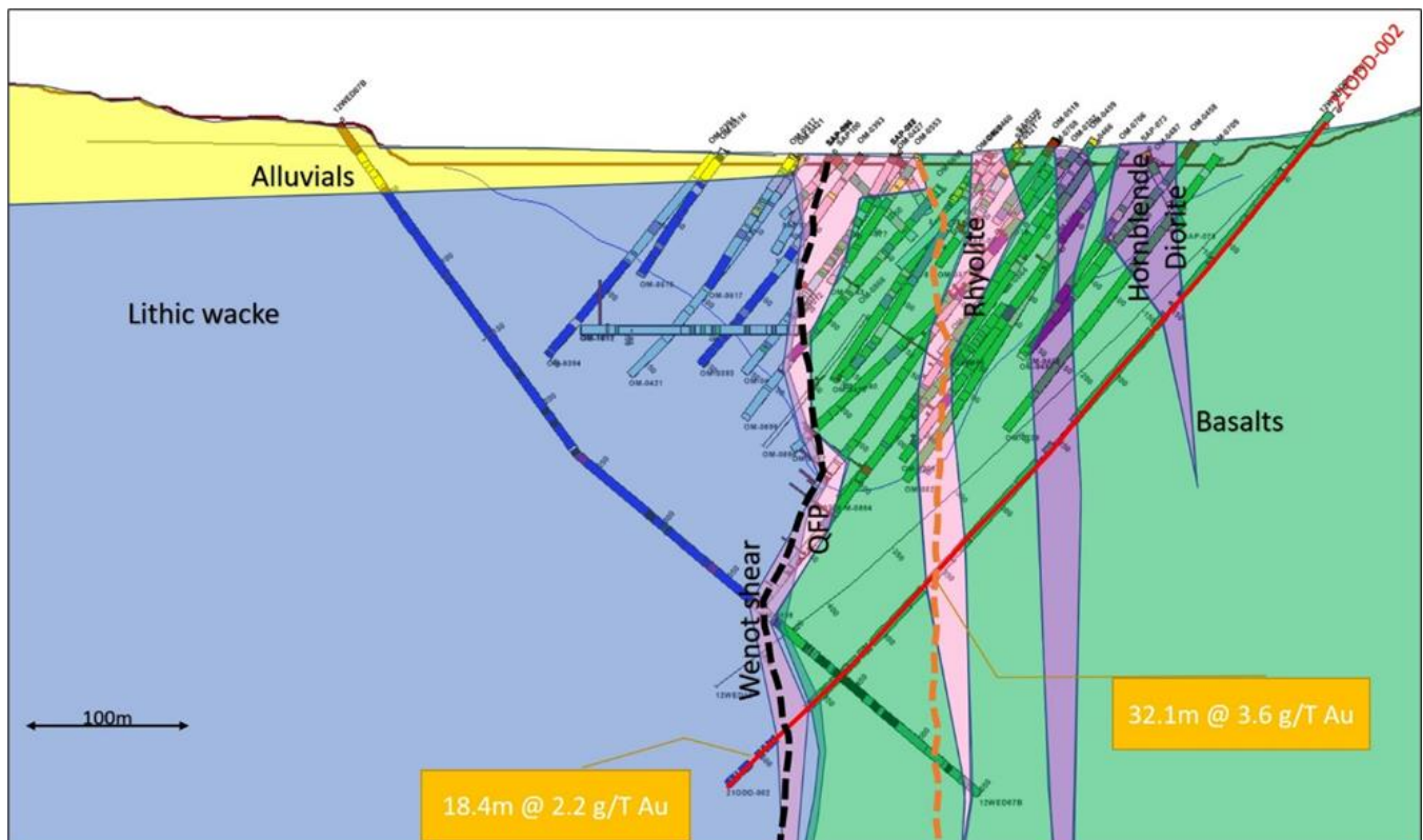
Figure 3: Section 5180 (looking west) showing geology and prominent intercepts of hole 21ODD-002 (526 m end-of-hole).
