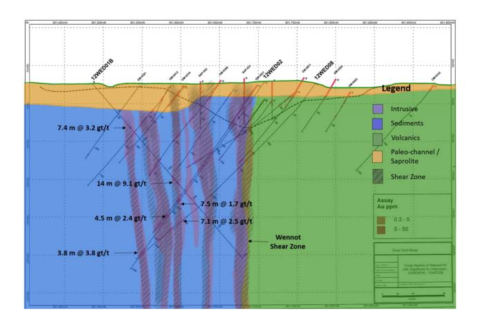
Figure 3: Cross section of holes 12WED04, 12WED05 and 12WED03B.
